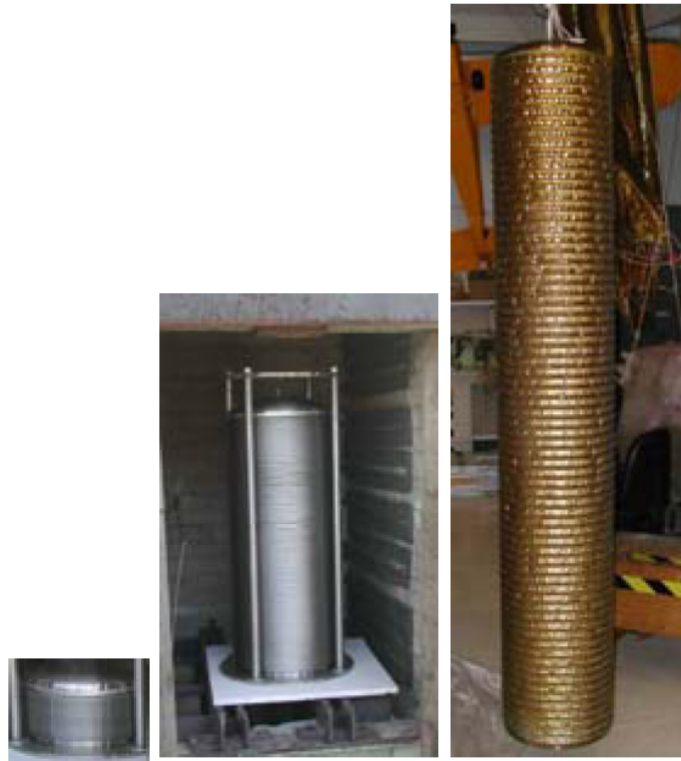
Figure 5.5: Proof of concept metallic bellows, tested at JPL.
