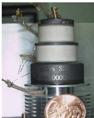
Figure 5.11: High temperature vacuum triode including heater, cathode, grid, and anode.
