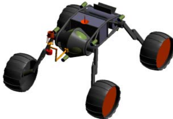
Figure B.1: Conceptual design of the Venus Rover CAD model with wheels deployed, perspective view (visualization by Shawn Krizan).
