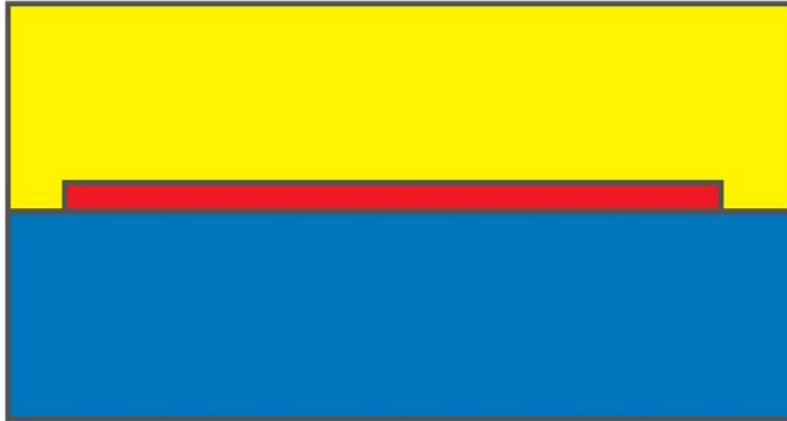
Figure 4.19: Cross section of the flux plate. The yellow material is a 1 cm thick low conductivity material, the red slab is a 1 mm thick copper plate, and the blue is high conductivity, conformable material with a thickness of 1 - 2 cm.
